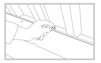
e. Insert the 13mm self-tapping bolts and washers and hand tighten to the chassis.
