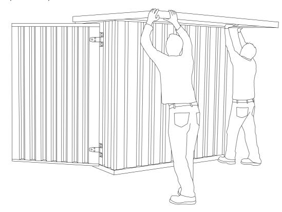
c. Once in position, pull the roof cap so that it locks into position all the way around.
