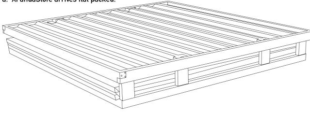
b. Undo and remove the 4 retaining nuts with your 19mm socket spanner (retain these for future use incase you want to return the store to its original flat-pack form).
