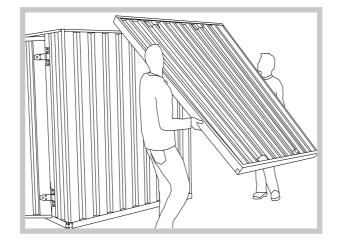
b. Slide the roof panel into position.
