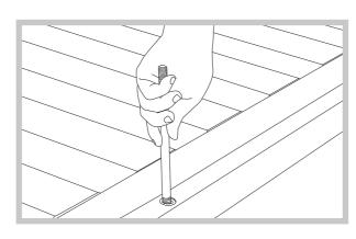
f. Remove the retaining bolts (retain these for future use in case you want to return the store to its original flat-pack form) and the final panel.
