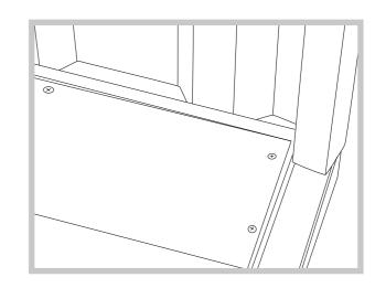
c. Butt the panel up against the chassis edge.
