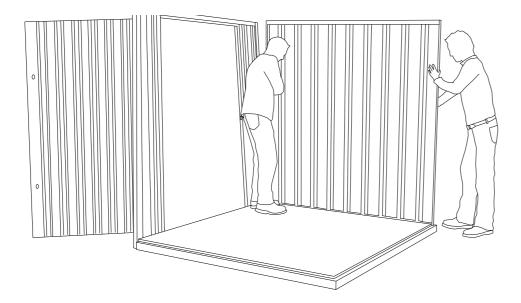
b. The wall panels should inter-lock.
