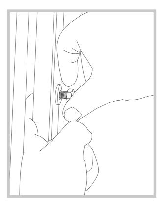
d. Insert the 13mm bolts & washers into the captive nuts and hand tighten.
