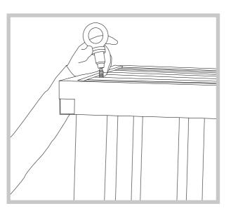
f. Outside attach the lifting eyes (with their rubber washer) to the end of the lifting rods.
