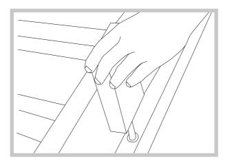
d. Remove the spacer protective blocks (retain these for future use incase you want to return the store to its original flatpack form).
